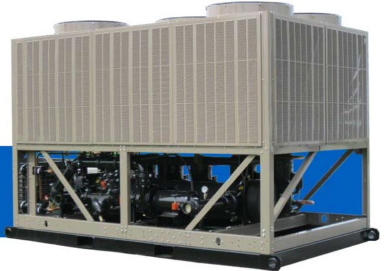
Resolute Industrial's York® brand Air Cooled Scroll Compressor Chiller package is self-contained and engineered to provide flexible, temporary chilled fluid for commercial and industrial air conditioning and process cooling applications. The chiller package is permanently mounted on a rugged steel tubular frame with fork-pockets for easy maneuvering, and features a single-point power connection and integral pump package.
